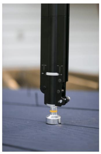
board installation, the absence of fastener versatility and the affordability and lack of flexibility in the deck fastening tools in use today. Installing decking at speeds up to 5X faster than current methods, the CAMO Drive tool allows the user to attach their own drill and stand up (get off their knees) while using any one of the three most popular methods of securing decking: Clips, Edge screws or Face screws.
